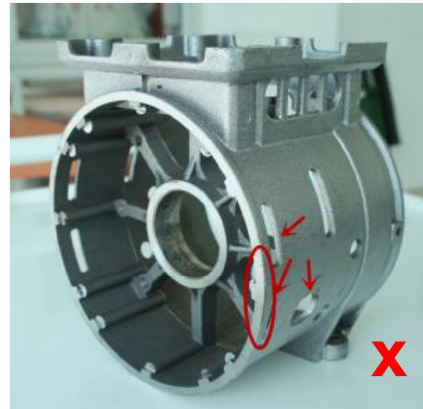
BRAND B: Shell edge and heat radiation holes are thin, have potential of cracking
