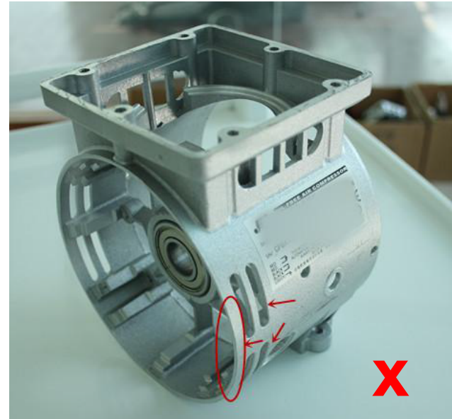
BRAND J: Shell edge and heat radiation holes are thin, have potential of cracking
