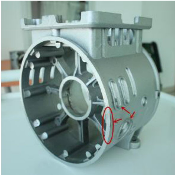
Pureflow Shell edge and heat radiation holes are Thickened, minimize the rate of cracking
